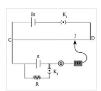
(iii) Balancing length l<sub>1</sub> is determined when key K<sub>2</sub> is open. According to principle of potentiometer.
